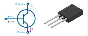
A bipolar transistor has terminals labeled base (B), collector (C), and emitter (E). A small current at the base terminal can control or switch a much larger current between the collector and emitter terminals.
