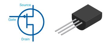
For a field-effect transistor, the terminals are labeled gate, source, and drain, and a voltage at the gate can control a current between source and drain.
